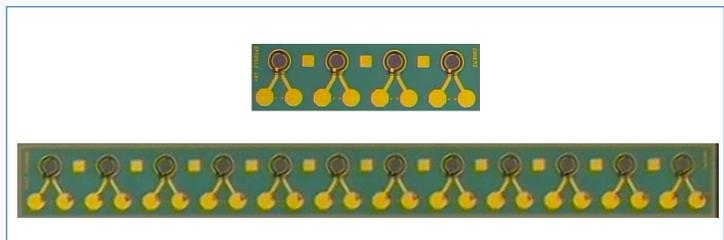
Cosemi's SPD2012-x is a mesa-structured, GaAs-based PIN photodiode offering high responsivity, low dark current and low capacitance for high bandwidth, high performance optical receiver designs. The SPD2012-x comes in a 1x4 and 1x12 array.
